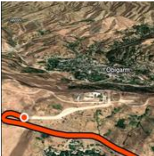
GPS Screenshot 1 (Elevation: 1,617 m): Highlights a sharp curve requiring reduced speeds and traffic management measures.
